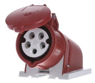
Wall socket TwinCONTACT 16A, 5p, 6h, 400V, IP44 - Wallmounted CEE-socket CEE-Socket 16A 31
