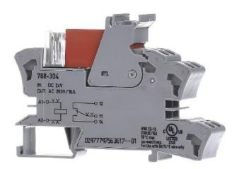
Switching relay DC 24V Type of electric connection Spring clamp connection, Rated control supply voltage Us at DC 24 ... 24V, Voltage type for actuating DC, Drive, polarization Polarized, Drive, switching attitude Mono stable, Number of contacts as normally closed contact 0, Number of contacts as normally open contact 0, Number of contacts as change-over contact 1, Type of switch contact Simple contact, Complete with socket, Degree of protection (IP) IP20, Width 15mm, Height 54mm, Depth 86mm
