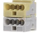
Bus coupler terminal light gray yellow screwed. 243-212 Number of clamping points 8, Cable diameter 0.6 ... 0.8mm, With actuating levers, Other color, Rated voltage 100V, Rated current 6A, Suitable for solid conductors, AWG range 22 ... 20, 4-wire socket terminal for Individual soldering pins for KNX Ø 0.8 mm pitch 5.75 mm 2-pin
