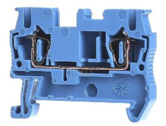
Tension spring terminal 0.08-4qmm B=5.2mm bl - Feed-through terminal block 5,2mm 24A ST 2,5 BU
