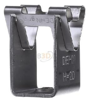
Conductor holder StSt for Rd 8mm H 20mm - Holder for lightning protection 207 019
