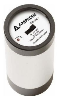
Sound level calibrator - Environmental measuring device SM-CAL1
