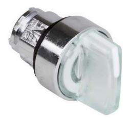
Illuminated selector switch 3st.button,ws for LED-M. -Short thumb-grip actuator white IP66 ZB4BK...
