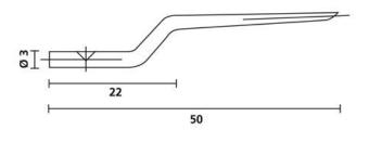
Replacement mandrel NA-0/1 DORNE, type of accessory=spare part, for easy mounting of any type of grommet on cables and lines. Simply slide the spout onto the spikes. Squeeze the pliers and pull them over the cable. Close the pliers, the spout is in place. For easy and safe use, we recommend using Hellerine as an assembly aid (see Chapter 2.3).
