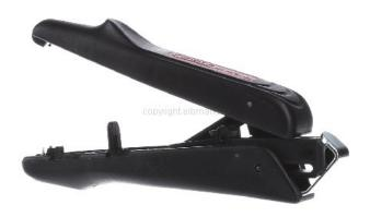
Duo-Stripper 12 0048 Stripping area diameter 4 ... 28mm, stripping area cross-section 0.5 ... 6mm², notch depth adjustable, round cut, stripping and stripping tool Duostripper, stripping and stripping with one tool, stripping for all common round cables from 4-28mm diameter, stripping Automatic adjustment to the conductor cross-section of 0.5-6qmm
