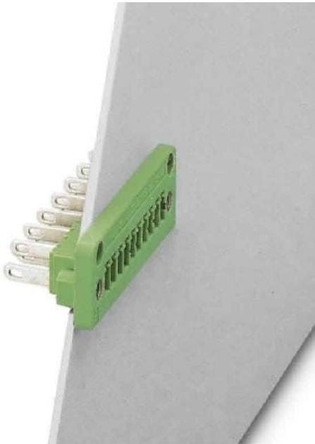
**Bushing housing 160V,8A,3.81mm,4p - Fixed connector for printed circuit DFK-MC1,5/4-GF-3,81**
