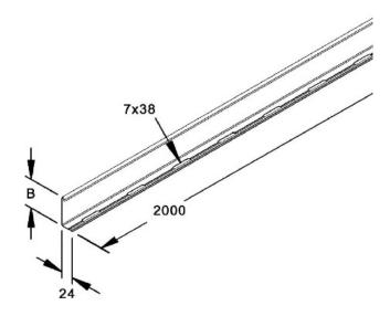
Separator galvanized - Separation profile for cable tray 3000mm RW 60
