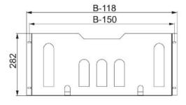
Metal plan pocket for door 800 NSYSDP8M Circuit diagram pocket design, material metal, suitable for housing width 800mm, color grey, RAL number 7035, height 282mm, depth 65mm, spacial metal document pocket. Width 800mm. For direct mounting on the door frame. Height adjustment every 25 mm on the door frame. Steel, painted. Gray RAL 7035.
