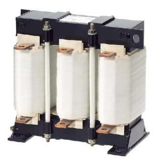
Mains choke frequency converter - Coil for low-voltage 3-pole 144A 480V 4EU2752-1UB00-0AA0
