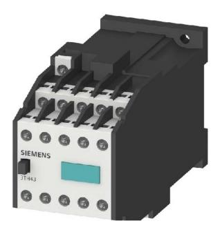
Auxiliary contactor DC bet. integrated variant - Contactor relay 0VAC 24VDC 2NC/ 8 NO 3TH4382-0LB4
