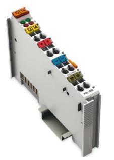
Digital output terminal 2-channel 24VDC 0.5A - Fieldbus digital module 0 In / 2 Out 750-506
