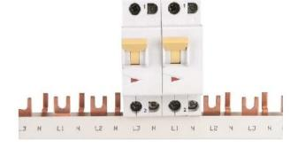
Number of phases 2, Number of poles 1, Pitch 0 mm, Cross-section 10 mm², Length 1000 mm, Width in division units 1, Rated continuous current lu 50 A, Execution of the electrical connection Pen, Isolated yes, Rated surge voltage 4 kV, Conditional rated short-circuit current lq 0 kA, Max. Rated operating voltage Ue 415 V, Rated short-time withstand current lcw 0 kA, Suitable for devices with neutral conductor no, Suitable for devices with auxiliary switch no
