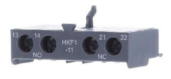
Auxiliary contact block 1 NO/1 NC Number of contacts as change-over contact 0, Number of contacts as normally open contact 1, Number of contacts as normally closed contact 1, Number of fault-signal switches 0, Rated operation current le at AC-15, 230 V 4A, Type of electric connection Screw connection, Model Top mounting, Mounting method Front fastening, Lamp holder None
