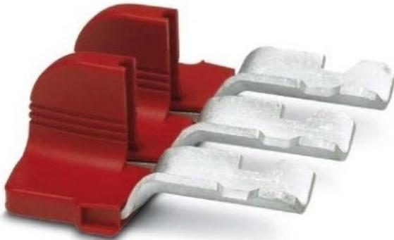
Insertion bridge EB 3-31/PT number of bridged terminals 3, rated current In 232A, isolated, pitch 31mm, color red, insertion bridge, pitch: 31mm, length: 78.4mm, width: 85.7mm, number of positions: 3, Red color
