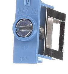
Terminal block WAK16/2 BL/V0 busbar thickness 3 ... 3mm, busbar width 10 ... 10mm, suitable for flat bars, terminal width 8.5mm, max. conductor cross section 16mm², suitable for round conductor connection, terminal block for neutral conductor busbar, nominal cross section 16 mm²
