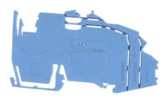
Busbar support plate for TS35 2009-304 number of poles 1, busbar support cannot be used as an end clamp, can be snapped onto TS 35, 1.5 mm thick, blue
