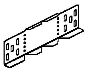
Reduction abs.angle - Length- and angle joint RAW 60.300
