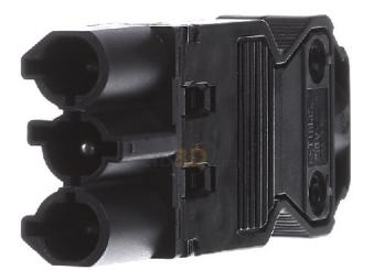
Plug part with strain relief - Connector plug-in installation 3x1,5mm<sup>2</sup> GST18I3S S1 ZR1 SW
