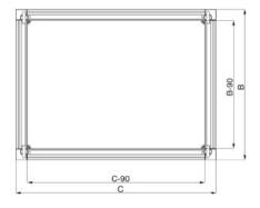
Top mounting module (switchgear cabinet), Width 400 mm, Height 300 mm, Depth 600 mm, Suitable for housing width 400 mm, Suitable for housing depth 600 mm, Material Steel, Type of surface powder-coated, Color gray, RAL number 7035, With cable entry no
