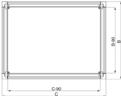
**Busbar compartment SF IP55 above, 300x1000x500mm - Top mounting module (switchgear cabinet) NSYTB...**
