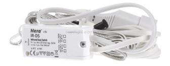
IR door contact switch 50612080241 base element, non-contact door contact switch for connecting lamp operating devices of protection class II, 3 m connection cable with Euro plug, 0.3 m switching cable with Euro coupling, 3 m sensor cable with K60 sensor head, switching function: the light switches on when the door is opened on and off again when the door is closed, including automatic safety shutdown of the lights after 30 minutes
