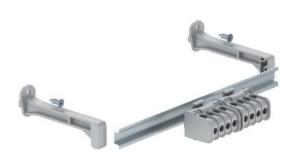
Terminal strip set with screw terminals KL-X16 06-16 rated current In 100A, rated voltage 450V, number of poles 5, number of terminal points per pole 4, other color, terminal strip set for the small distributors of the SDB series. The sets can be used to extend and equip empty small distributors of the SDB series
