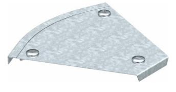
Bend cover for cable tray 150mm, Bend (angle) 45 °, Width 150 mm, Suitable for cable tray yes, Suitable for mesh cable tray no, Suitable for cable ladder yes, Fastening type Spagnolet, Hinges no, Suitable for function maintenance no, Material Steel, Stainless steel, stained no, Material quality other, Surface galvanized zinc-aluminum, Color without, Change of direction horizontal
