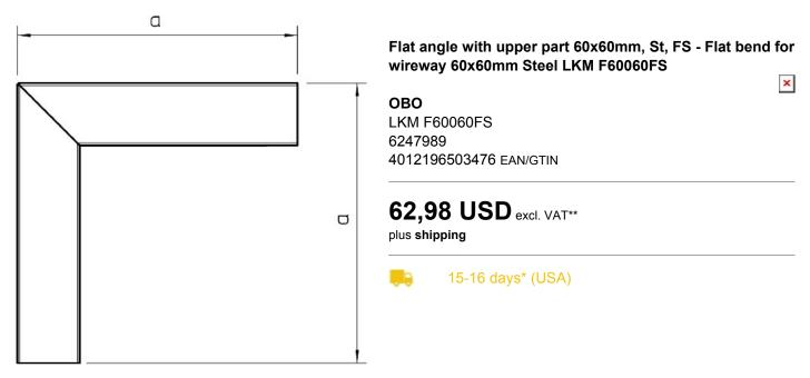
Flat bracket with upper part 60x60mm, St, FS LKM F60060FS Height 60mm, width 60mm, design lower part and upper part, angle 90 ... 90°, material steel, surface strip-galvanised, color other, type of fastening bottom perforation, flat bracket with upper part for changing the direction of the LKM cable routing ducts. Equipotential bonding is guaranteed between the lower and upper parts without any further aids.
