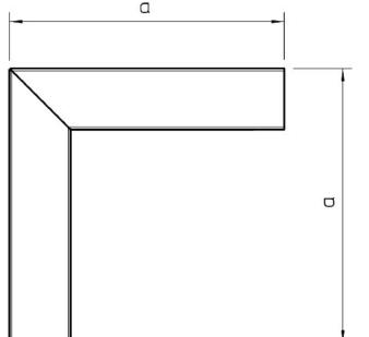
Flat angle with upper part - Flat bend for wireway 60x40mm Steel LKM F40060FS
