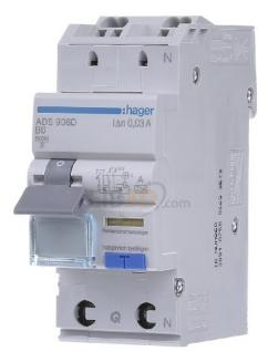
Residual current circuit breaker with line protection twopole B-6A 30mA ADS906D
