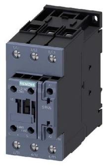
Contactor 22kW/400V, 1NO+1NC - Magnet contactor 51A 175...280VAC 3RT2036-1NP30
