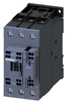
Contactor 18, 5kW/400V, 1NO+1NC - Magnet contactor 41A 175...280VAC 3RT2035-3NP30
