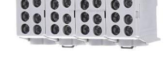
Rail terminal bar 4-p screw clamp Number of poles 4, Connection type Screwing, Mounting method DIN rail, Number of connections total 18, Number of connections < 6 mm<sup>2</sup> 0, Number of connections 10 mm<sup>2</sup> 0, Number of connections 16 mm<sup>2</sup> 10, Number of connections 25 mm<sup>2</sup> 8, Number of connections > 25 mm<sup>2</sup> 0, Contact safe
