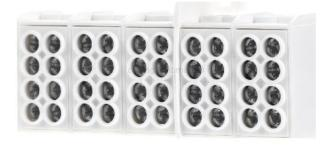
Power distribution block 5-p screw clamp Number of poles 5, Nominal current 80A, Connection type Screwing, Mounting method DIN rail, Number of connections total 20, Number of connections < 6 mm² 0, Number of connections 10 mm² 0, Number of connections 16 mm² 0, Number of connections 25 mm² 20, Number of connections > 25 mm² 0, Contact safe, Height 65,9mm, Width 102,4mm, Depth 45,5mm
